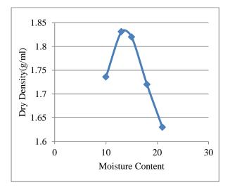
Fig. 3. Dry Density v/s Moisture Content of soil
