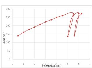
Fig. 8. Variation in Penetration (in mm) for soil reinforced with 0.6% Fiber
