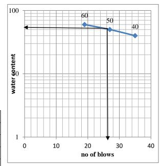
Fig. 1. Water Content v/s Number of Blows
