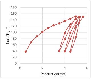
Fig. 4. Variation in Penetration (in mm) for unstabilised soil
