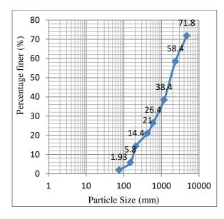
Fig. 2. Grain Size Distribution Curve
